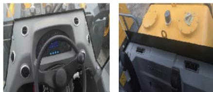
Repositioned vents throughout the cab keep fresh air flowing while improving the cab's heating, cooling.
