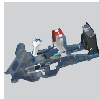
Load sensing steering maximizes machine performance by directing power through the steering system only when needed. When the machine is not steering, more engine power is available to generate rimpull, breakout and lift forces. Load sensing reduces horsepower draw by up to 8 percent, resulting in better fuel economy. Large-bore steering cylinders allow responsive maneuverability.
