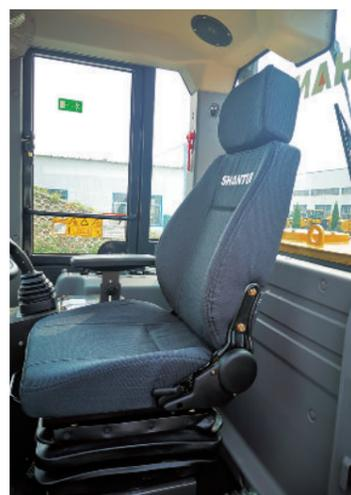
The vertically and horizontally adjustable suspension seat ensures the operator can work long days in comfort and with less fatigue.
